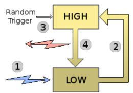
My understanding of how such a machine should operate is illustrated on the left. The machine is in its low-energy state. It is hit by a travelling disturbance (1) which imparts energy to it. This raises (2) the machine to its high-energy state. After a random delay (3), the machine falls back again to its low-energy state (4). In the process of so doing, the machine creates a fresh disturbance in the space around it, which travels outwards away from it.
