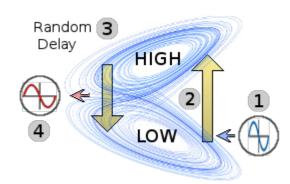
Thus the whole machine could simply be a twin-lobed complex dynamical system, which, when hit by an incident disturbance (1) is pushed (2) onto its upper lobe. Then, after an apparently random delay (3), it falls back to its lower lobe, releasing its excess energy as the emitted disturbance (4). Although the delay appears to be random, it is deterministic. It's just that the determinism is very complex, thereby creating an illusion of randomness.
